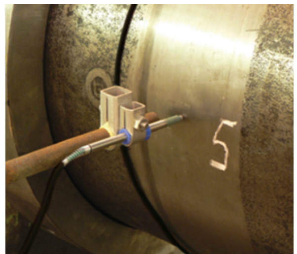
Closeup of Gauging Probe checking for deformation and strain on oil and hydrogen tanks
