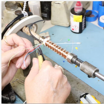
A transducer coil being wound by hand
