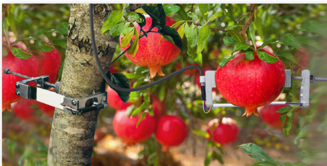
Dendrometry of a pomegranite using Solartron Sensors
