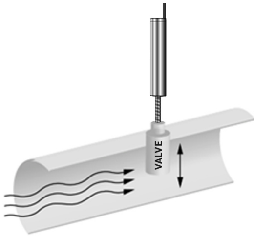
Gas flow testing using an LVDT
